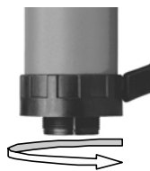
fig. 1 Screw lock ring fully onto pump.
