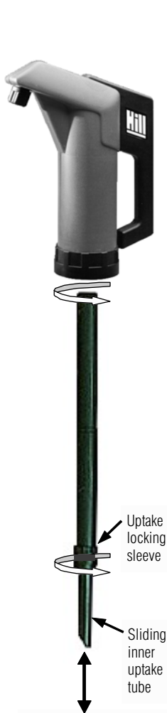
fig. 2 Fitting and adjustment of Telescopic uptake pipe
